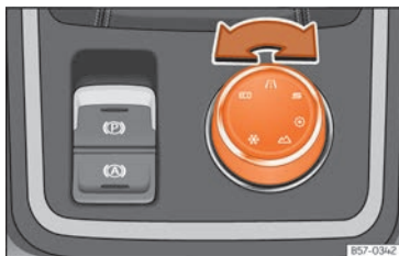
Fig. 277 Consola central: Mando rotativo [Driving Experience button].
